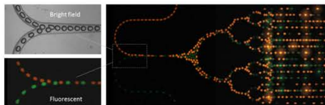
Fig. 3. Hybrid microfluidic chip channels: (left to right) 2:1 microfluidic combiner with droplets doped with two types of fluorescent markers emitting light at 521nm (green) and 580nm (orange), the 1:16 microfluidic divider and the chip detection zone as seen by the fluorescent microscope. The enhanced brightness of some droplets in the detection zones is due to the lensing effect of the micro lens array.
